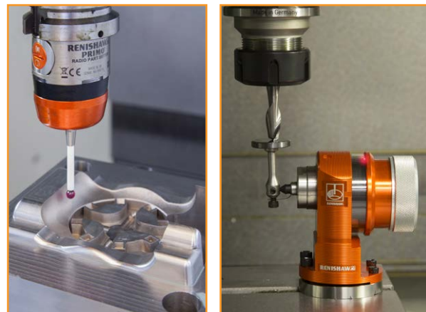
The images above show a Renishaw Primo Radio Part Setter (left) in use on an XYZ high-speed vertical machining centre whilst setting a 3D mould. The Primo Radio 3D Tool Setter (right) is used to automatically set tool lengths and diameters.
