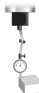
Part setting with a dial gauge
