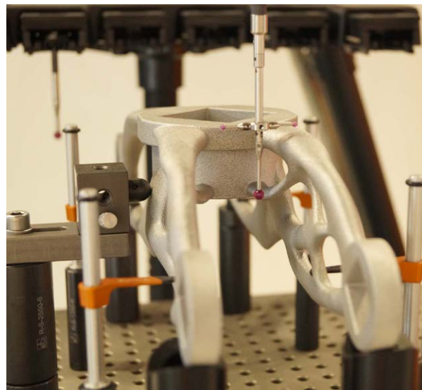
Figure 3: Bleu car hinge component being measured on a Renishaw Equator™ gauging system
