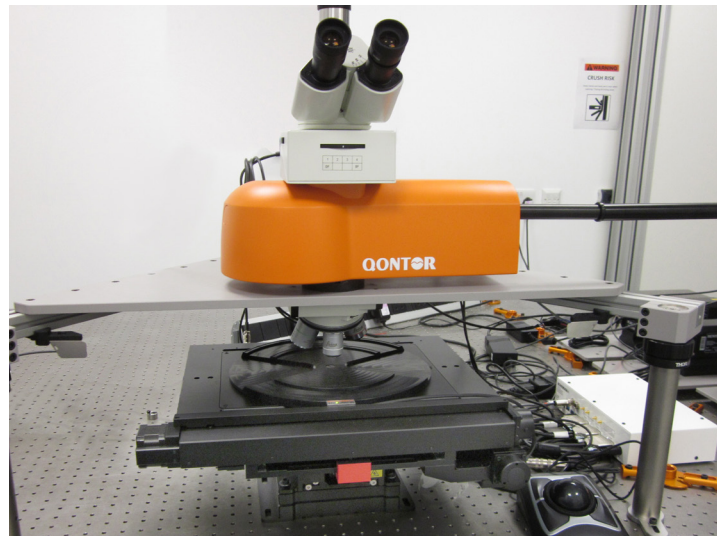
An inVia Qontor confocal Raman microscope is configured as a wide free-space microscope. Together, the Prior H112 and Renishaw MZ40 stages enable the complete inspection of 12" semiconductor wafers.
