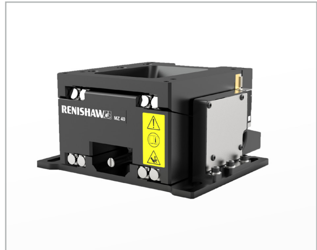
The MZ40 Z stage is equipped with a 100 nm resolution Renishaw encoder. This enables you to position it accurately and reproducibly anywhere within its 18 mm range of travel.
