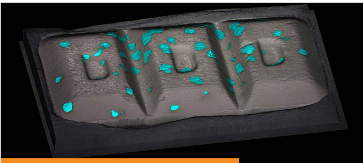
Raman image of a tablet showing the distribution of API (cyan).
